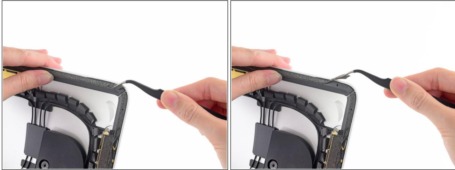
**⚠** Before you start placing strips, remove all of the old adhesive from around the perimeter of the rear enclosure.
