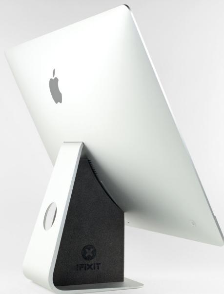
**i** With the hinge free to move, the iMac will be unbalanced and hard to work on. Repairs can be completed as shown, but are faster and easier with an [iMac service wedge](#).
