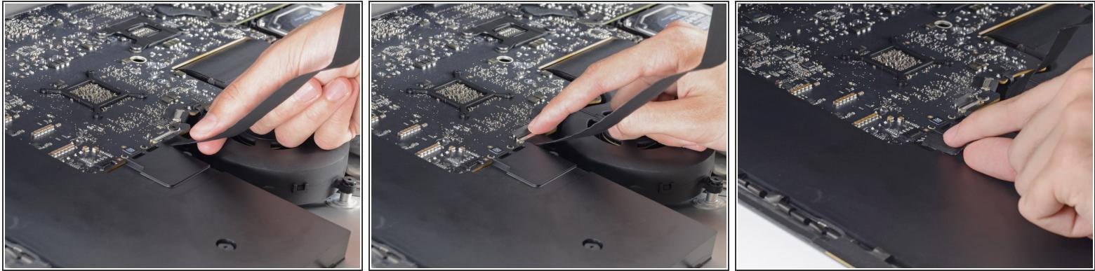
*(i) At this point it's a good idea to test your repair, in order to make sure your iMac works properly before you seal it back up. Follow the next three steps to temporarily reconnect the display cables and boot up your iMac prior to pulling the protective film off the adhesive strips.*
