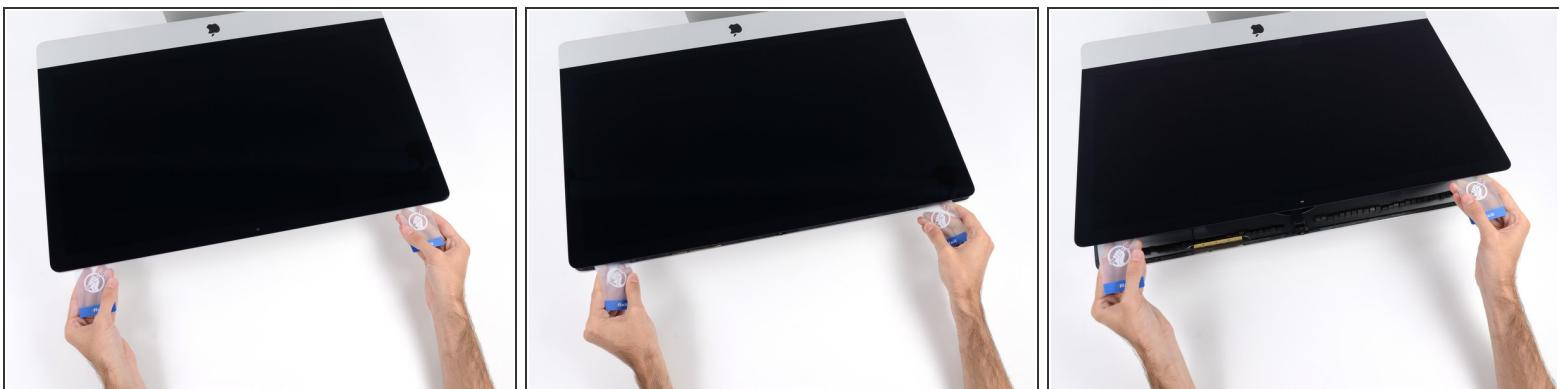
⚠ Only lift the display a few inches—it is still attached to the iMac by data and power cables.
