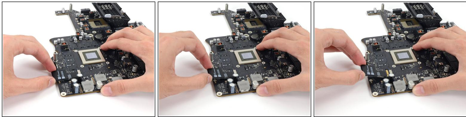
! To avoid damaging its socket, do not lift the end of the AirPort/Bluetooth Card excessively.
