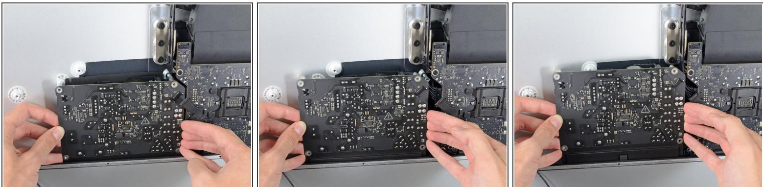
**⚠ Do not attempt to remove the power supply from the case; it is still attached to the logic board by two cables.**
