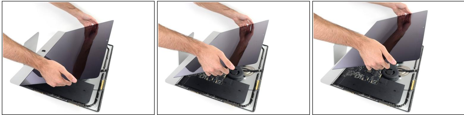
**⚠** Be very careful handling the display—it's big, heavy, and made of glass. The display has fragile edges. Avoid lifting the display by the corners.
