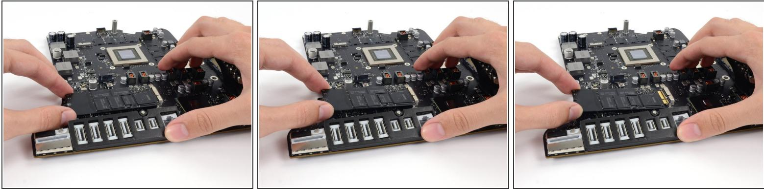
! To avoid damaging its socket, do not lift the end of the SSD excessively.
