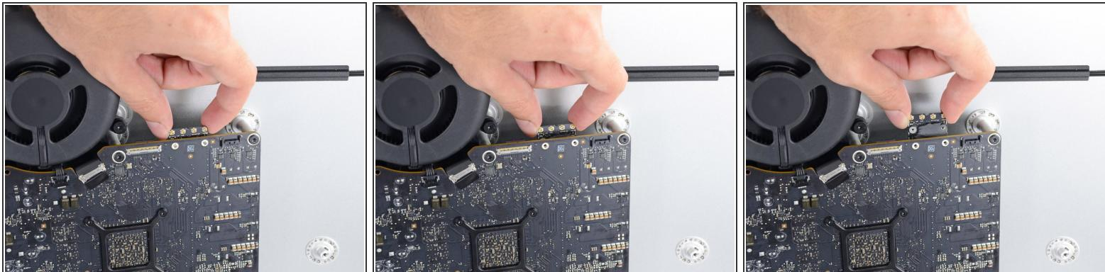
⚠ To avoid damaging its socket, do not push the end of the AirPort/Bluetooth Card away from the logic board excessively.
