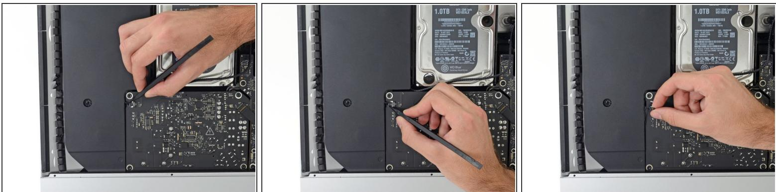
**⚠** Be careful not to touch any solder joints on the back of the power supply. Capacitors may be charged enough to give you a dangerous shock.
