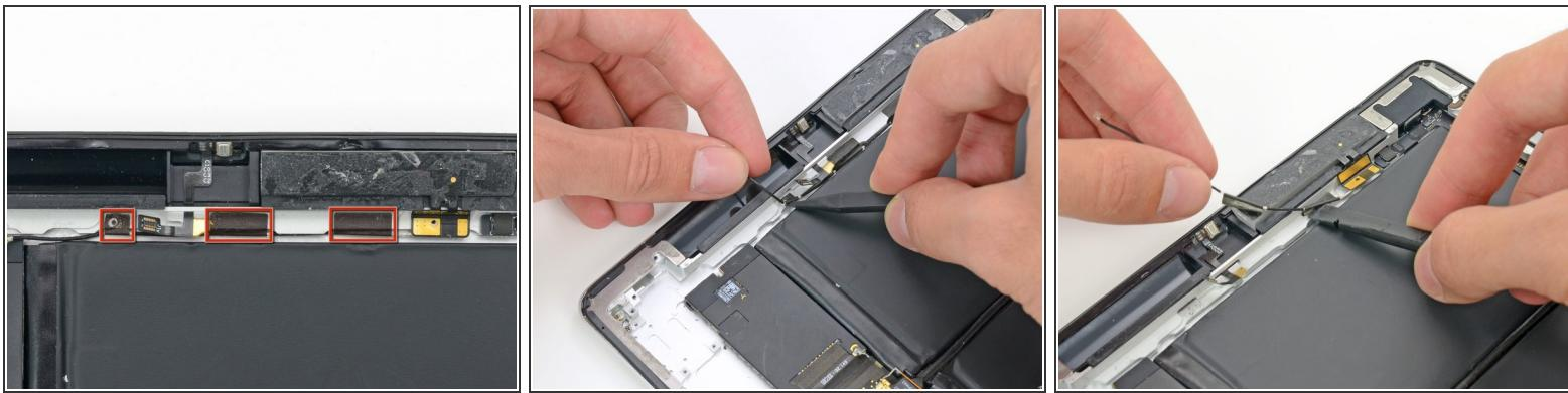
**⚠** In this step you will remove the three pieces of tape securing the right cell antenna cable to the rear case.
