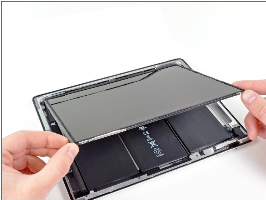
*(i)* In order to work on the iPad's innards, we need to flip the LCD back out of the case.
