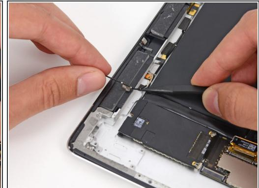
! In this step you will remove the two pieces of tape securing the cellular data antenna cable to the rear case.
