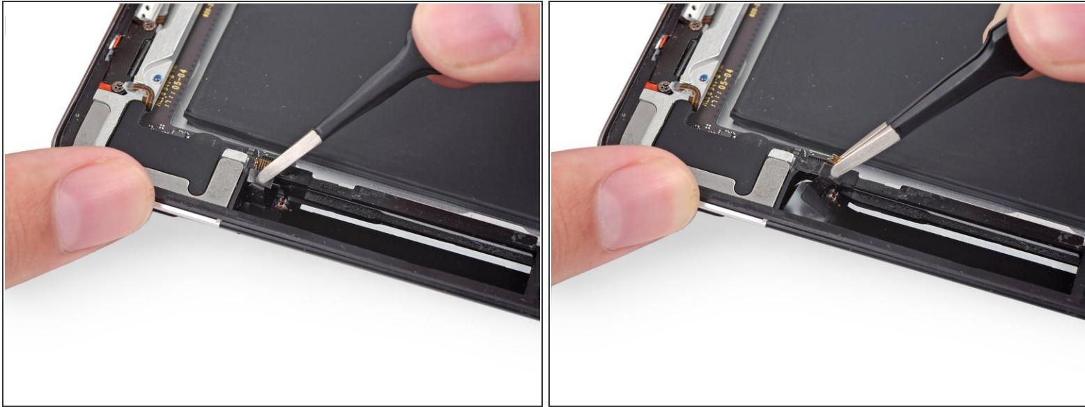
ⓘ Removing the GPS antenna can be very challenging. The method shown in the following steps is one that worked for us. However, you should only follow this guide if you are replacing the GPS antenna with a new one, as this could irreparably damage the antenna.
