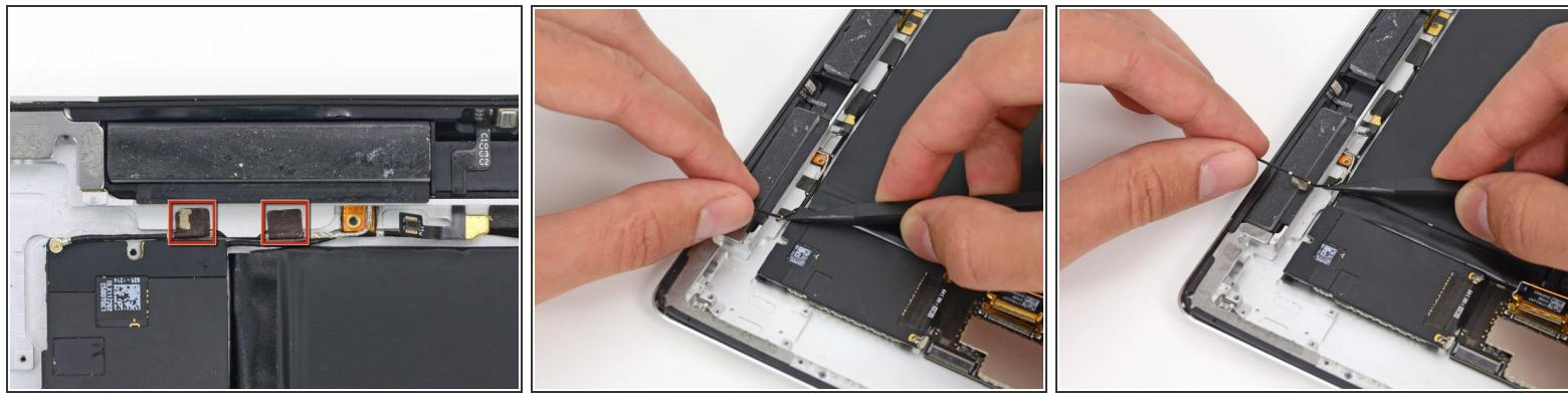
**⚠** In this step you will remove the two pieces of tape securing the cellular data antenna cable to the rear case.
