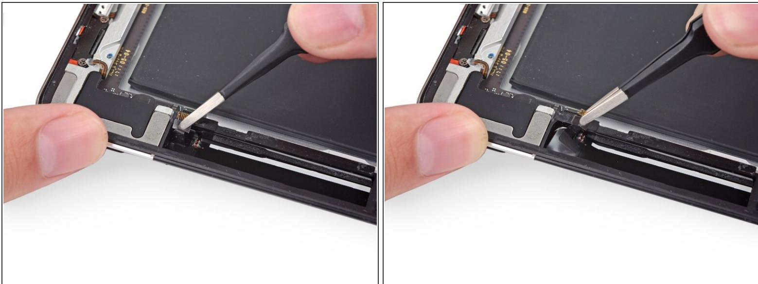
*(i)* Removing the GPS antenna can be very challenging. The method shown in the following steps is one that worked for us. However, you should only follow this guide if you are replacing the GPS antenna with a new one, as this could irreparably damage the antenna.
