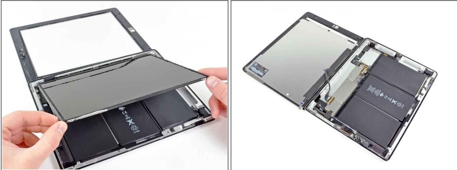
*(i)* The front panel ribbon cables are connected beneath the LCD. To access them, you'll need to temporarily flip the LCD over and out of the way.
