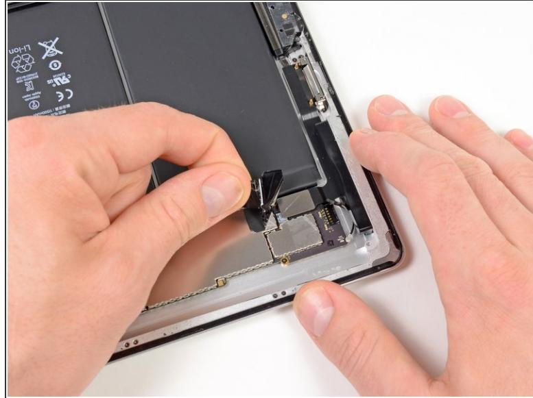
*(i)* If present, remove the pieces of electrical tape covering the Wi-Fi antenna, speaker cable, and dock connector cable.
