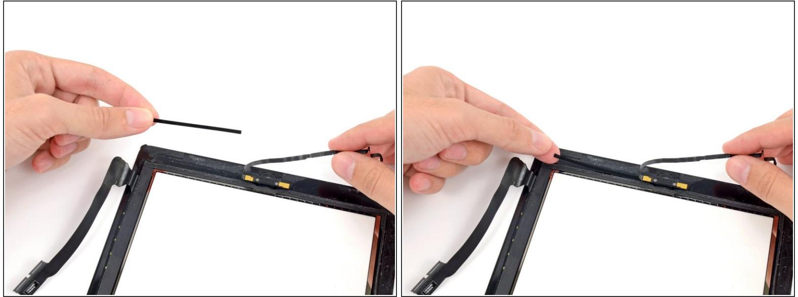
*(i)* It is recommended to lift the home button ribbon cable aside while placing the next adhesive strip.
