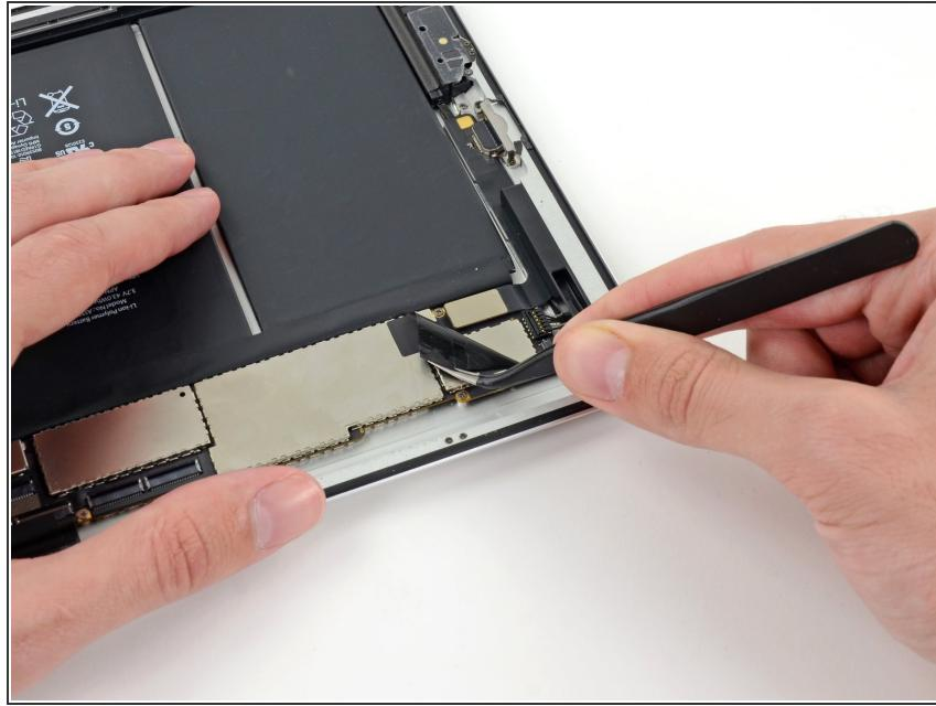
ⓘ If present, remove the piece of electrical tape covering the Lightning connector cable.
