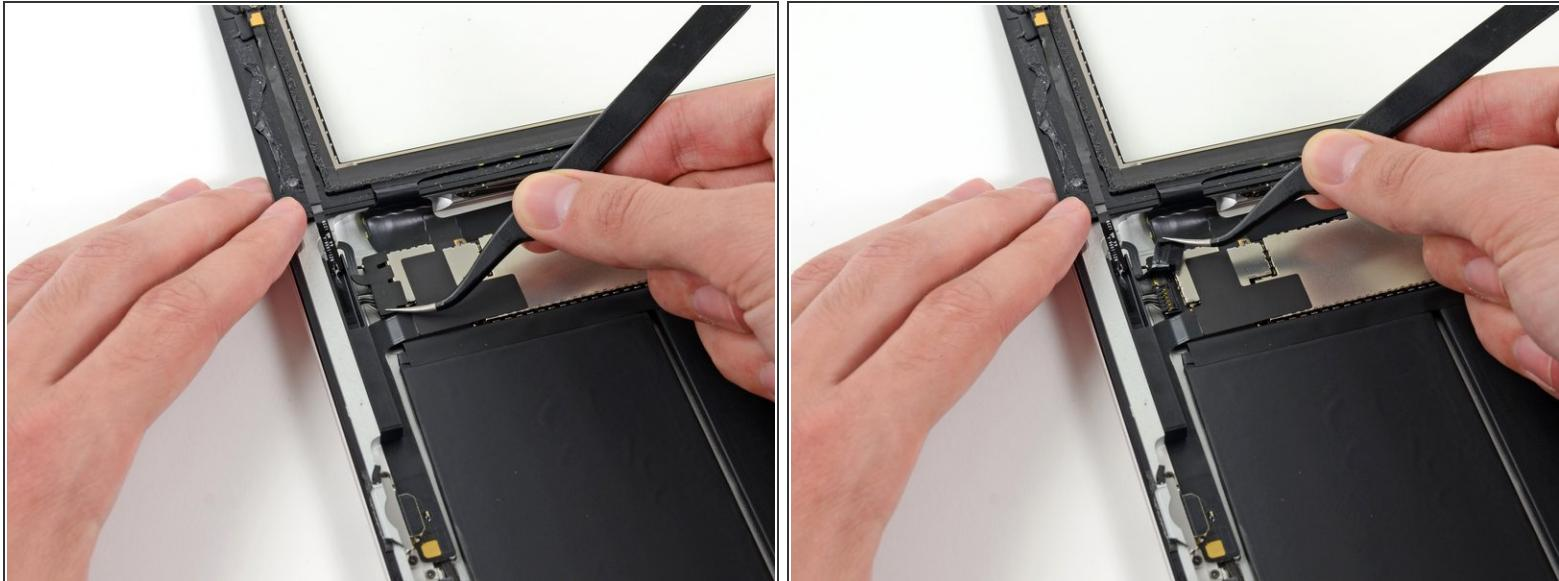
*(i)* If present, remove the piece of electrical tape covering the Wi-Fi antenna, speaker cable, and home button ribbon cable.
