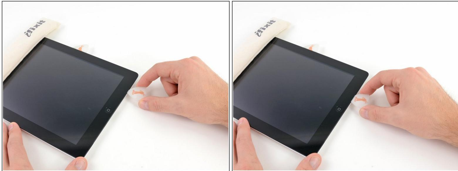
**⚠** This step requires you to move the opening pick along the bottom right edge of the front panel. The Wi-Fi antenna is very close to the corner and is easily severed if the adhesive is released improperly.
