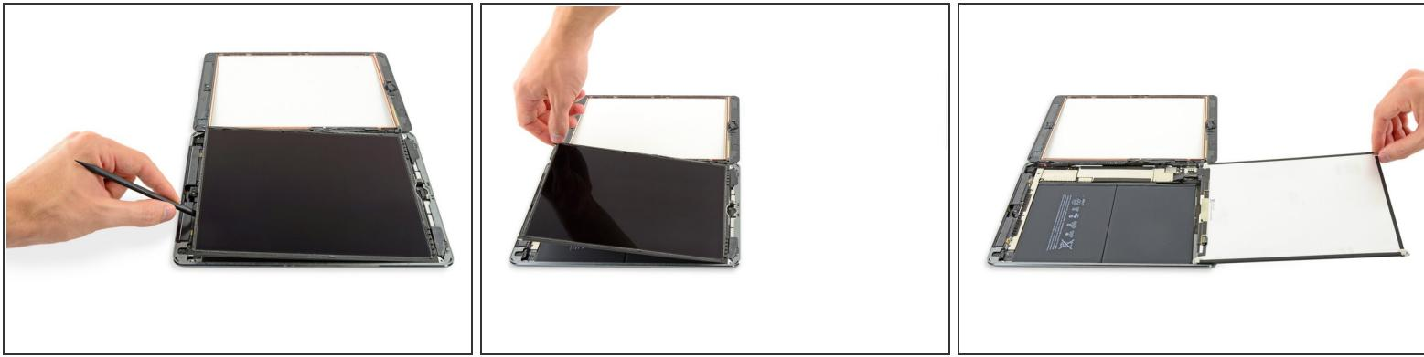
**⚠** Do not attempt to fully remove the LCD. It is still connected to the iPad by several cables at the home button end. Lift only from the front-facing camera end.
