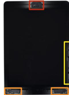
**(i)** While the iPad looks uniform from the outside, there are delicate components under the front glass. To avoid damage, **only** heat and pry in the areas described in each step.
