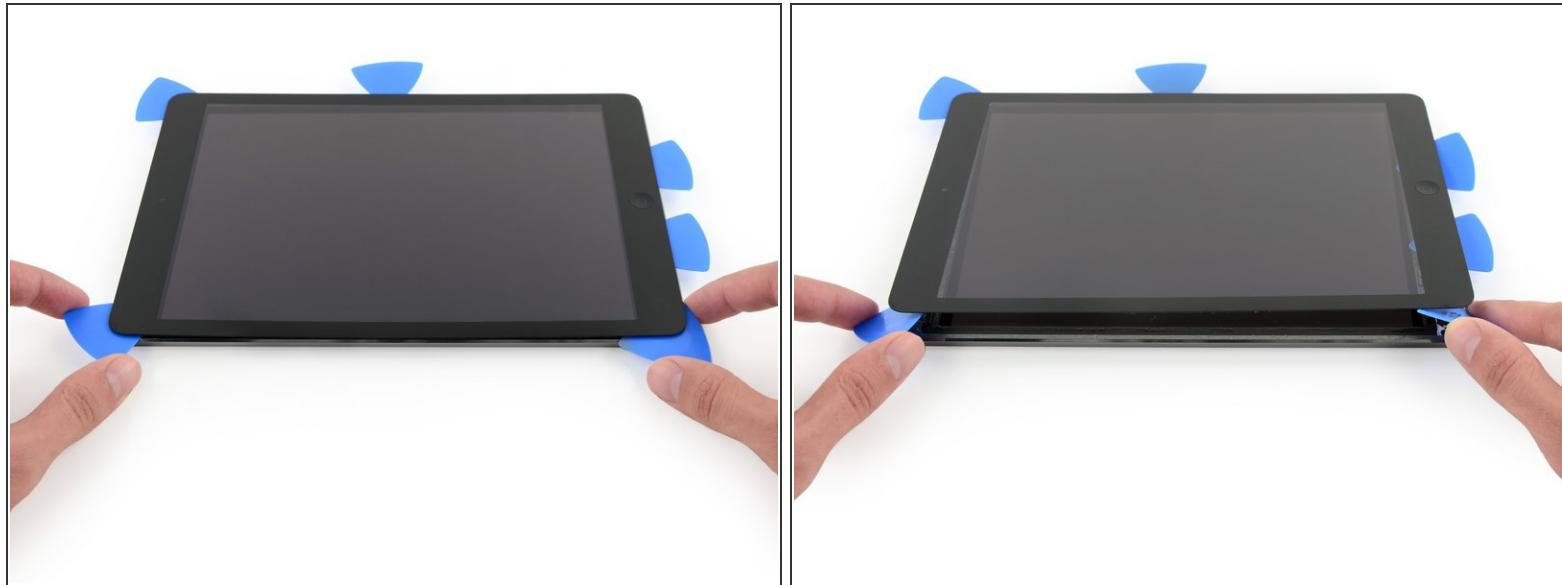
**⚠️ Be very careful with this step.** Take your time and ensure the adhesive is hot and soft, and that you've been through all of the adhesive with an opening pick. Don't be afraid to stop and reheat.
