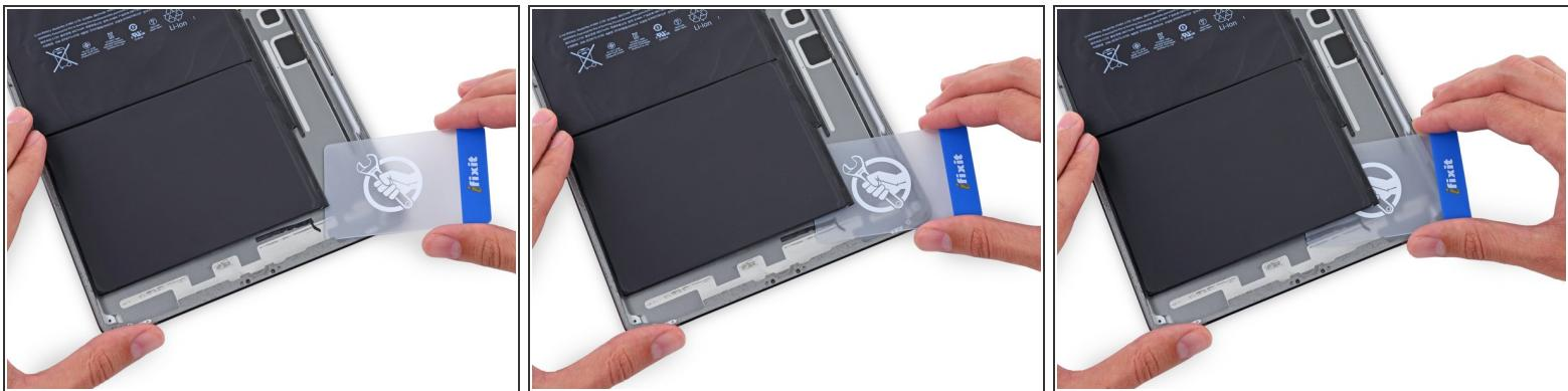
**⚠** Throughout the following procedure, you'll be sliding thin plastic cards between the battery and rear case of the iPad, to separate the adhesive securing the battery. Be careful to keep the cards as flat as possible to avoid bending the battery, which may damage it and cause it to release dangerous chemicals.
