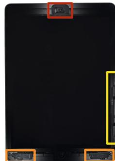
**(i)** While the iPad looks uniform from the outside, there are delicate components under the front glass. To avoid damage, **only** heat and pry in the areas described in each step.
