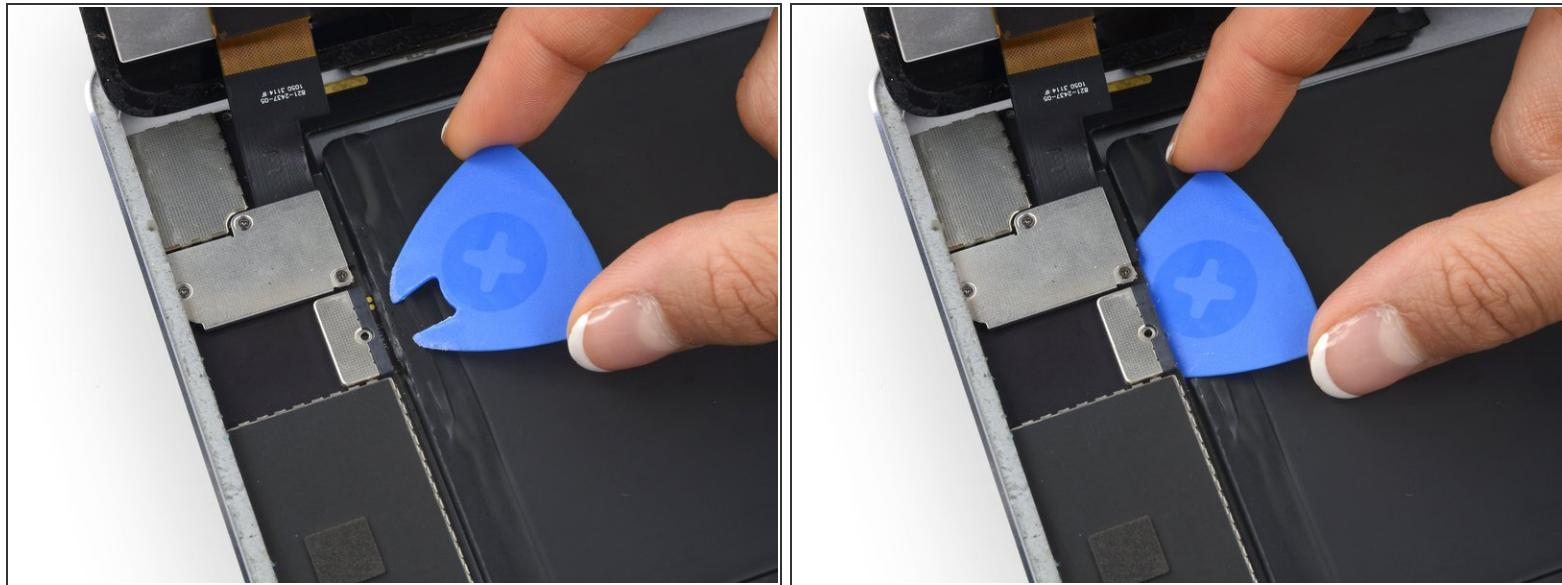
*(i)* To reduce the risk of a short, you can use a battery isolation pick to disconnect the battery.
