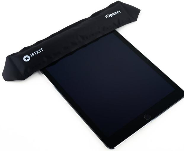
**i** The following steps involve using an iOpener to soften the adhesive holding the front panel assembly in place. When using the iOpener, be sure to heat it in the microwave for no more than 30 seconds.
