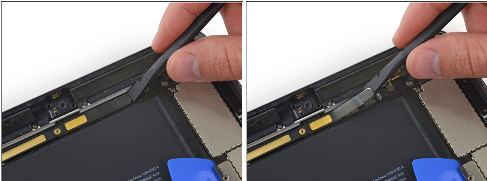
**⚠** The following steps involve disconnecting many press connectors from their sockets on the logic board. When disconnecting these cables, be sure to pry up only on the connector, and not the socket itself.
