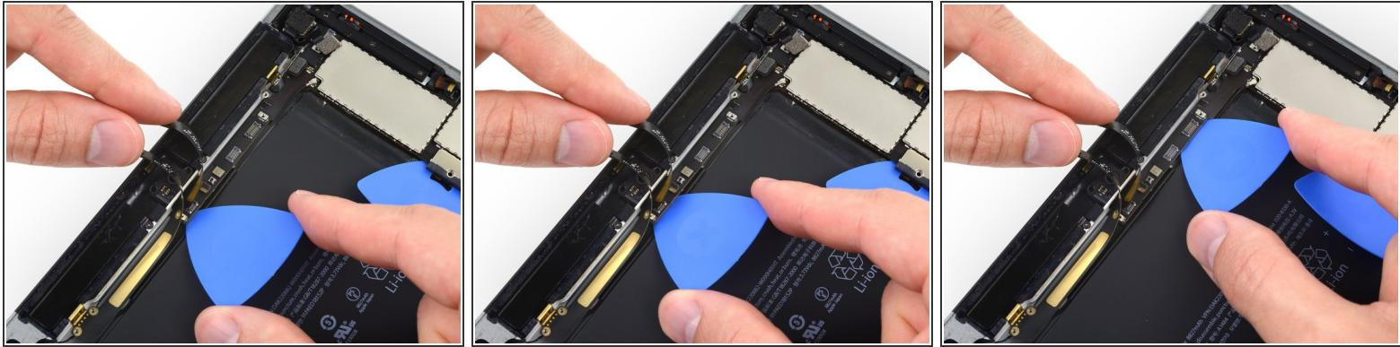
**⚠** As you complete the next few steps, prying adhesive securing the logic board in place, always start by testing gently to see if the adhesive is softened. If not, reheat the iOpener and reapply it to the back of the rear case.
