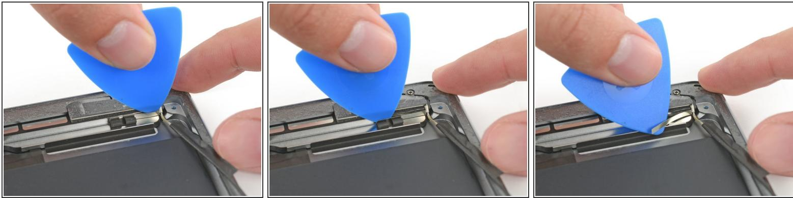
ⓘ There is a bracket crimped onto the antenna cable that is adhered to the speaker enclosure. The adhesive must be severed in order to extract the antenna.
