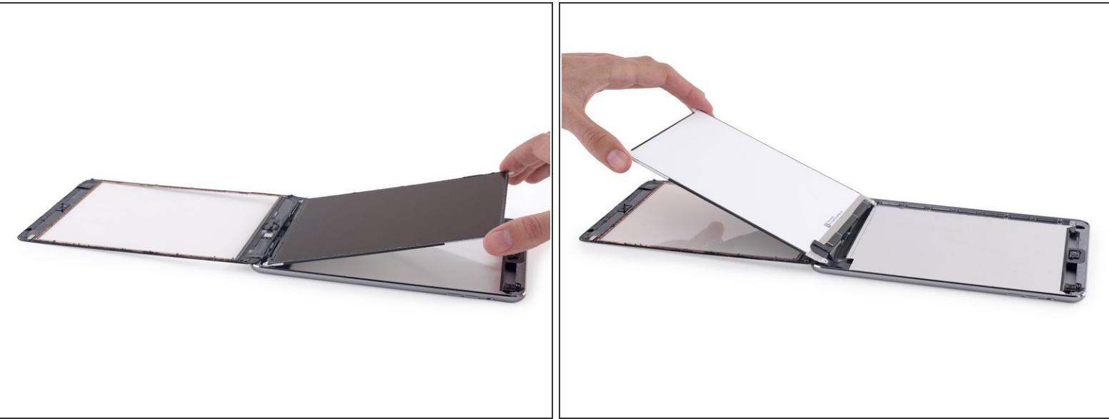
**⚠** Do not attempt to fully remove the LCD. It is still connected to the iPad by several cables at the home button end. Lift only from the front-facing camera end.
