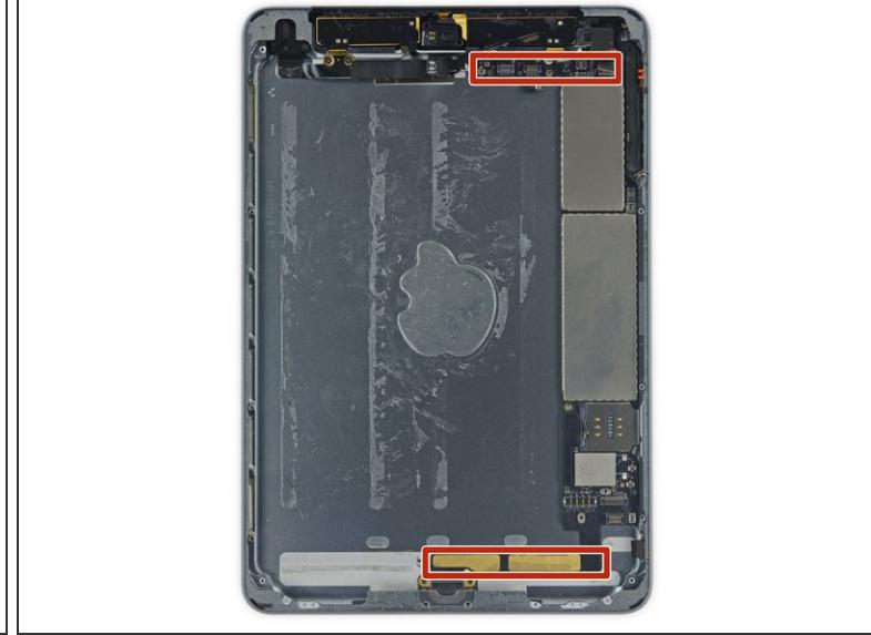
**ⓘ** The logic board is held in place by two strips of adhesive.
