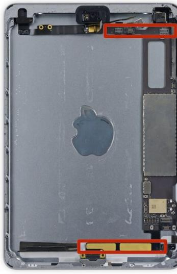
*(i)* The logic board is held in place by two strips of adhesive.
