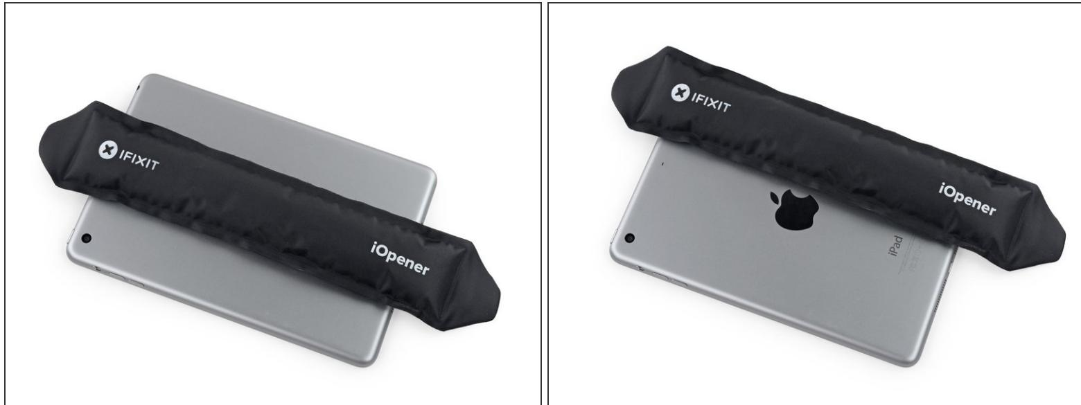
*(i)* The battery is held to the iPad case with some adhesive that will need to be heated in order to be separated.
