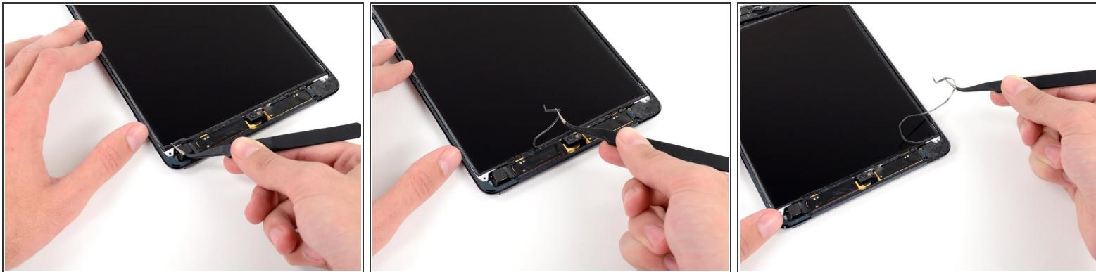
ⓘ A thin strip of foam tape on the LCD frame is covering a piece of tape connecting the LCD to the panel beneath it. To proceed, you'll have to break and peel up some of the foam tape to expose the tape hidden beneath.
