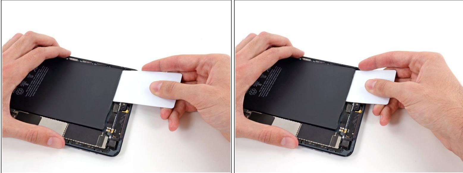
**⚠** Throughout the following procedure, you'll be sliding thin plastic cards between the battery and rear case of the iPad, to separate the adhesive securing the battery in place. Be careful to keep the cards as flat as possible to avoid bending the battery, which may damage it and cause it to release dangerous chemicals.
