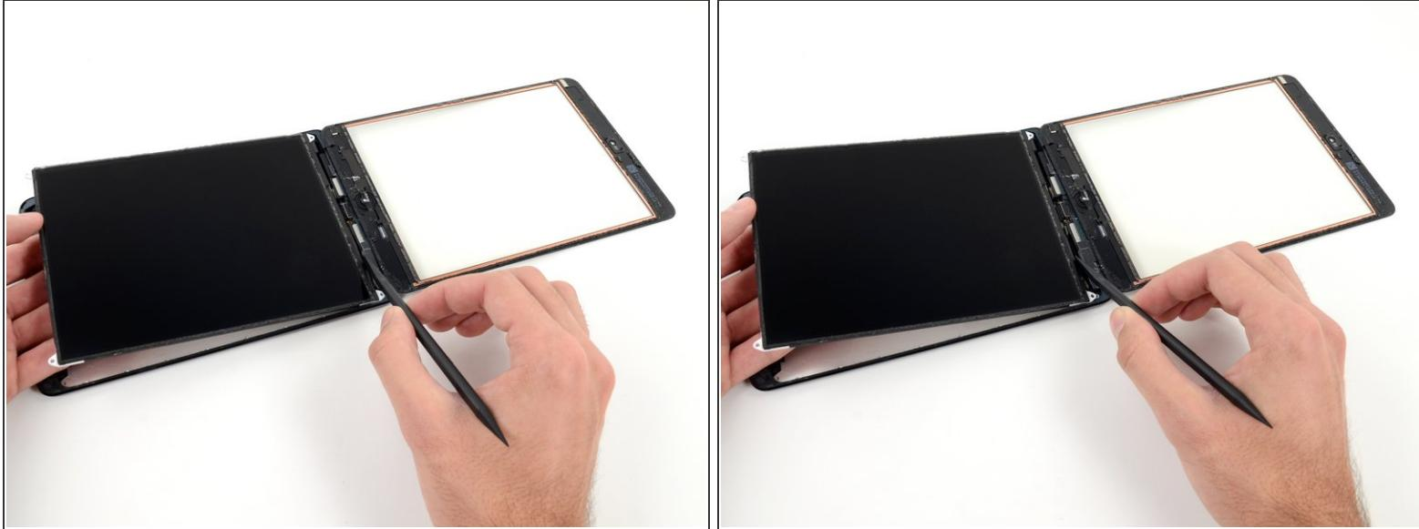
*(i)* Two wide strips of tape connect the LCD to the speakers.
