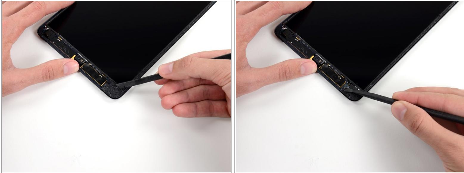
*(i)* The top left LCD screw may be covered by adhesive tape from the front panel.
