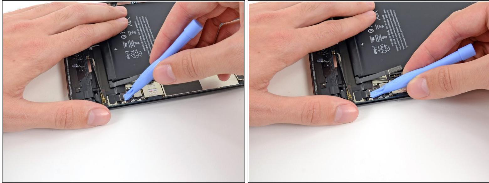
**⚠** Be very careful to pry evenly on the digitizer connector, and not on the socket at all. The socket and connector are very delicate and if you damage either, your digitizer won't work.
