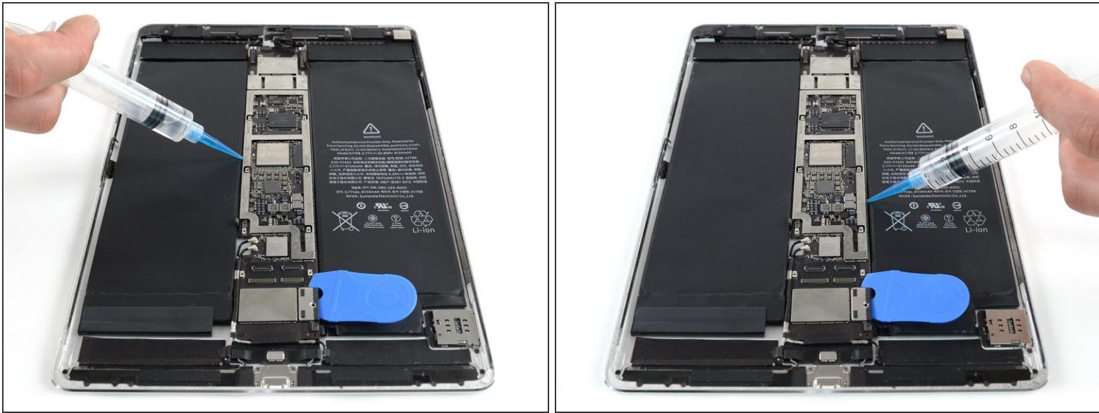
*(i)* The adhesive that holds down the logic board is very strong. To remove the board, you must first weaken the adhesive using either a solvent, or heat.
