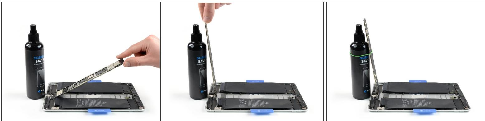
**⚠** In this step, don't fold back the logic board to more than a 100° angle. Some connectors are still attached to it and can be damaged.
