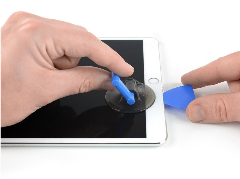
**i** If your iPad's screen is badly cracked, wear skin and eye protection. Cover the screen with a smooth layer of clear packing tape to contain glass shards and help the suction cup adhere. Alternatively, use a strong piece of tape (such as duct tape) and [fold it into a handle](#).
