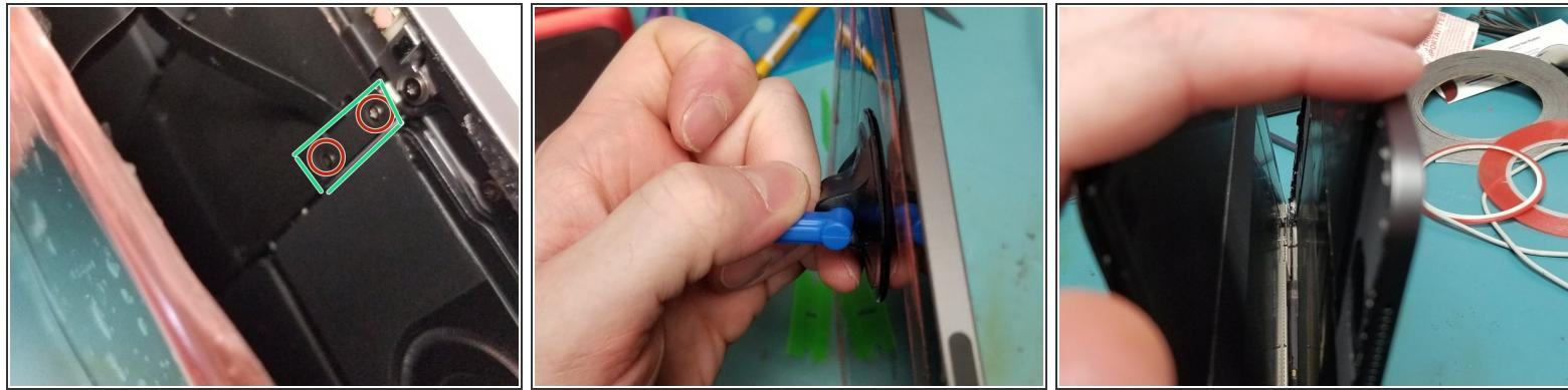
**⚠ Do not rip the screen off!! Cables are very short will cause internal Damages!!!**
