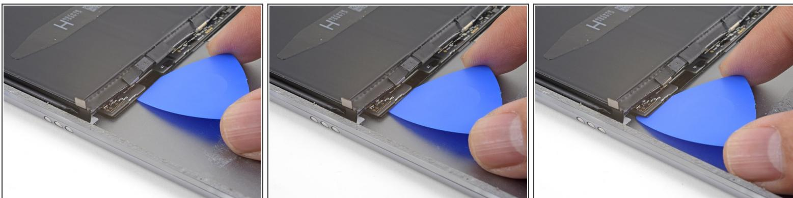
ⓘ The end of the mid-battery circuit board closer to the Smart Connector is held down with adhesive.
