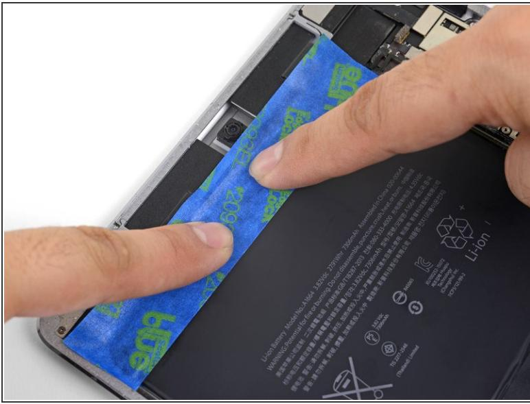
*(i)* The next four steps detail how to mask off the iPad in preparation for the liquid adhesive remover. The tape will help block and absorb excess liquids, keeping major components safe.
