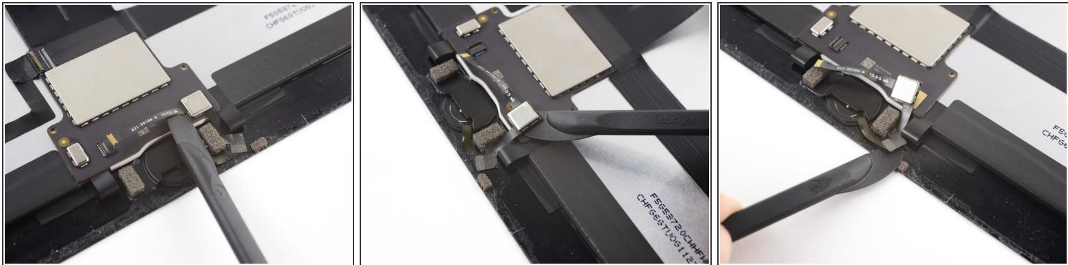
**⚠** The home button's ribbon cable is **very** fragile. If it gets damaged, or if the home button has to be replaced, Touch ID will no longer function.
