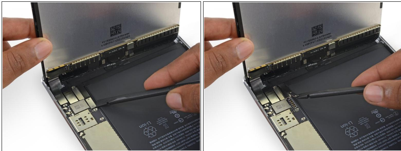
**⚠** When disconnecting any press connectors from the logic board, be sure to lift the connector straight up to avoid ripping the socket off the board.
