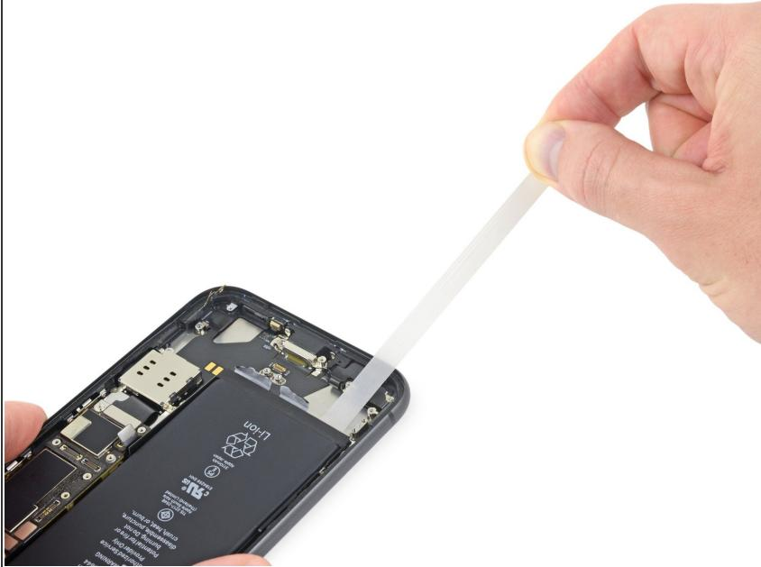
**i** In the following steps, you'll pull each tab to *slowly* stretch out the adhesive underneath the battery. The adhesive releases as it stretches.
