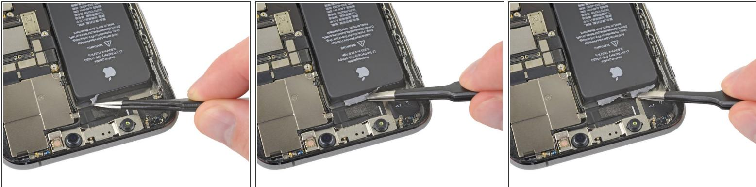
**⚠** The top pull tabs lie very close to the [Face ID sensors](#). If damaged, Face ID can only be repaired by Apple, so work with care. Don't touch the lenses with your fingers.
