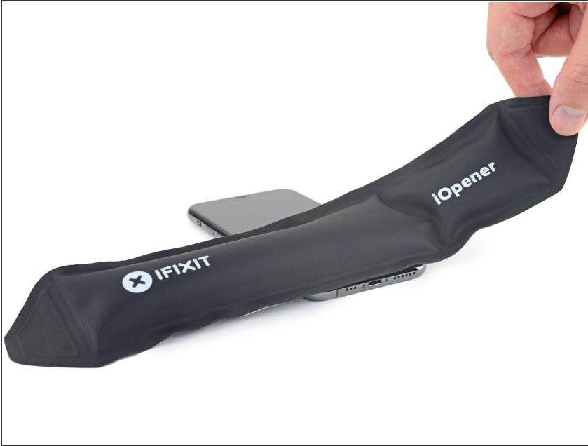
ⓘ Heating the lower edge of the iPhone helps soften the adhesive securing the display, making it easier to open.
