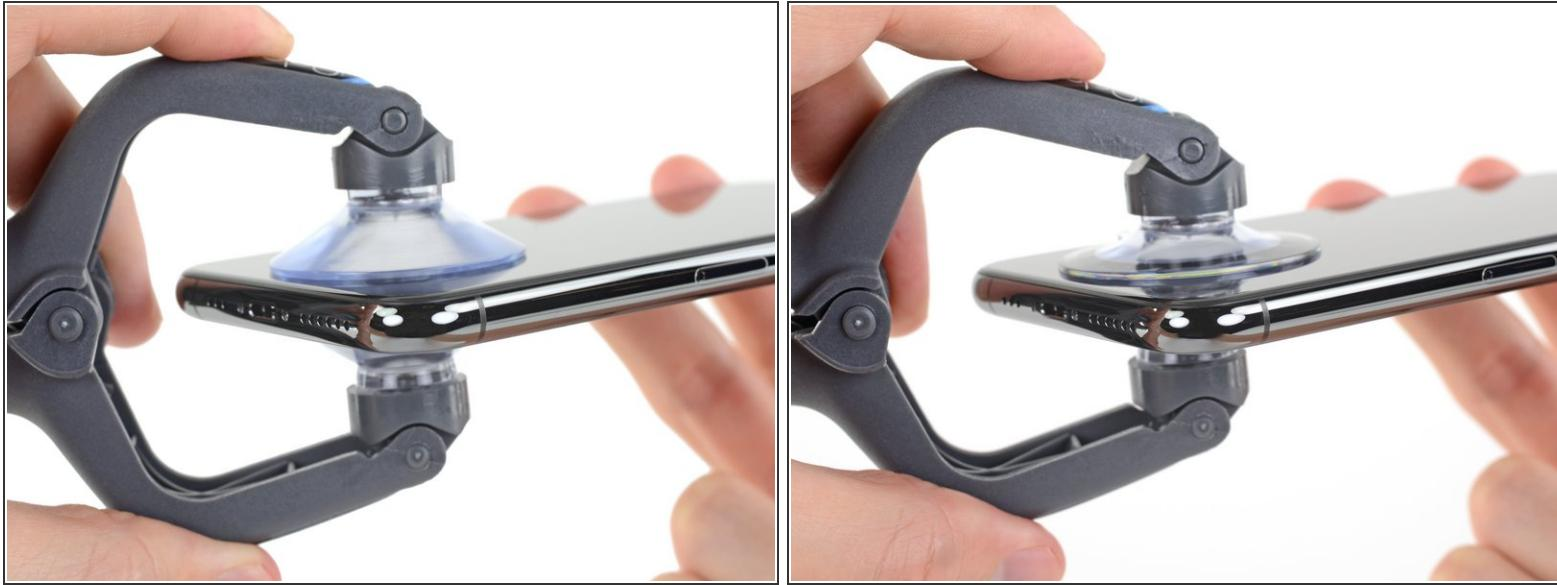
*(i)* The next two steps demonstrate the iSclack, a handy tool that we recommend for anyone doing frequent repairs. **If you aren't using the iSclack, skip down two steps for an alternate method.**
