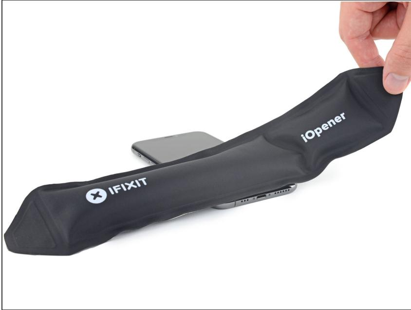
**i** Heating the lower edge of the iPhone helps soften the adhesive securing the display, making it easier to open.
