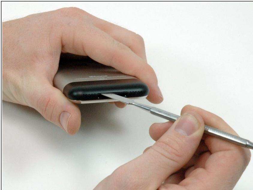
⚠ Be sure to slide the metal spudger between the dock connector and the antenna cover, and not into the dock connector itself.
