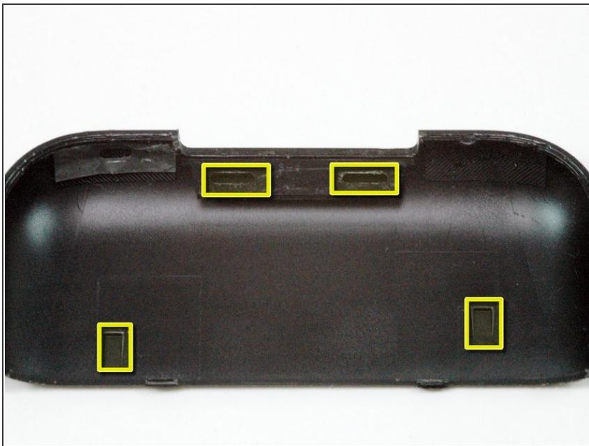
ⓘ This image shows the two tabs and two catches located on the underside of the antenna cover. The two tabs at the top of the image must be pushed towards the black cover to release them.
