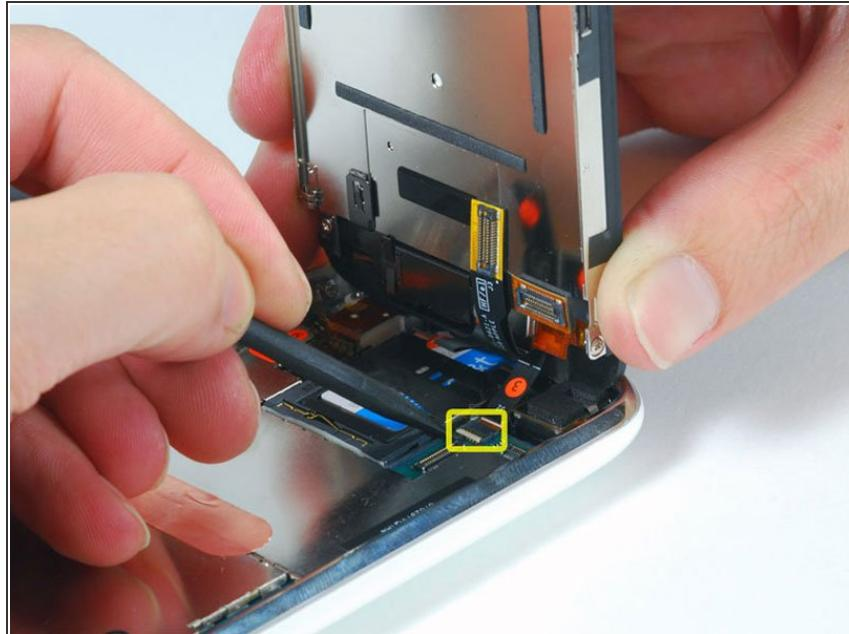
**⚠** Please note: You may find on some non-American (Chinese, European) versions of the 3G that the flip up plastic tab does not exist. In this case you would slide the ribbon cable towards the screen until it is removed. When you assemble it, you would apply pressure to the ribbon to insert it back into the ribbon "socket."
