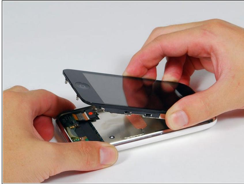
*(i)* The display assembly is still connected to the iPhone by several cables, so don't try to remove it entirely just yet.
