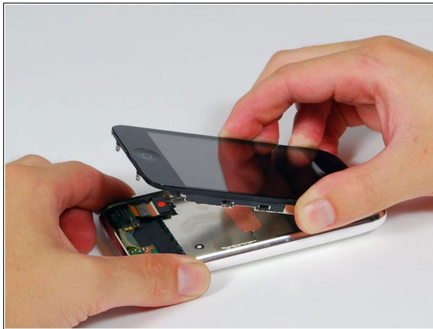
**⚠** The display assembly is still connected to the iPhone by several cables, so don't try to remove it entirely just yet.
