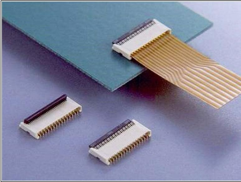
**⚠** Ribbon cable "3" is held in place by a FPC style connector. You must unlock this connector before sliding the ribbon cable out. The locking mechanism is on the opposite side of where the cable is inserted - it swivels upwards 90 degrees. Use a plastic spudger to lift the locking mechanism.
