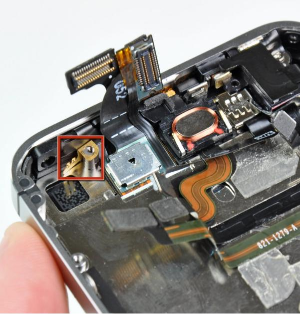
⚠ Be sure not to lose the small grounding finger for the rear facing camera near the power button.
