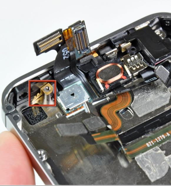
⚠ Be sure not to lose the small grounding finger for the rear facing camera near the power button.
