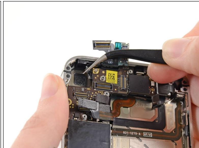
**ⓘ** If present, remove the piece of tape covering a Phillips screw near the power button.
