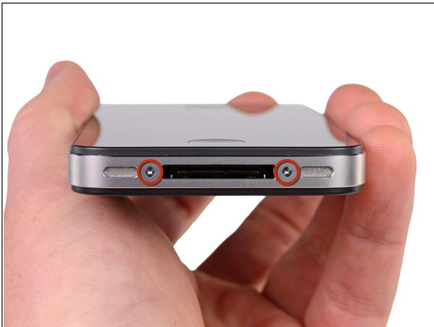
**⚠** Before you begin, discharge your iPhone battery below 25%. A charged lithium-ion battery can catch fire and/or explode if accidentally punctured.
