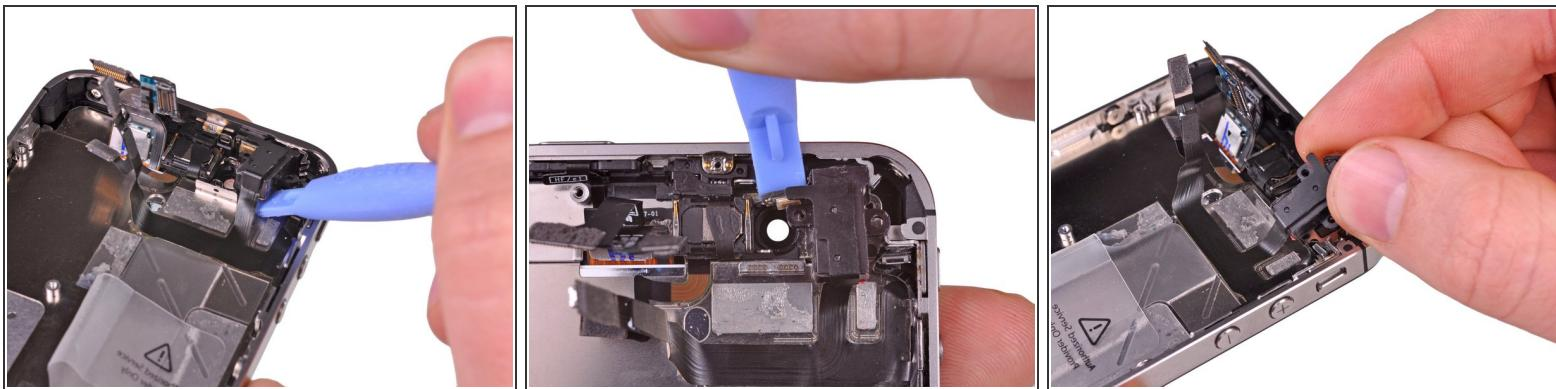
**⚠** In this step, be careful not to remove the headphone jack without first separating the top microphone from the upper case, as they are connected by a fragile flex cable.
