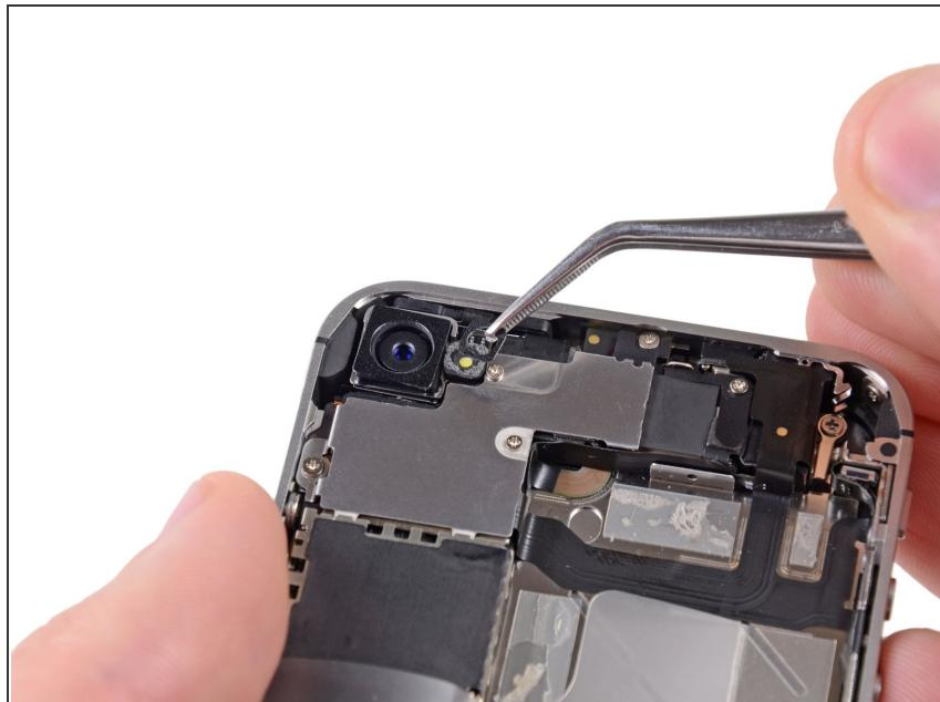
! Be wary of the outer plastic ring located on top of the rear camera's flash assembly. It can be easily displaced if not removed during disassembly.
