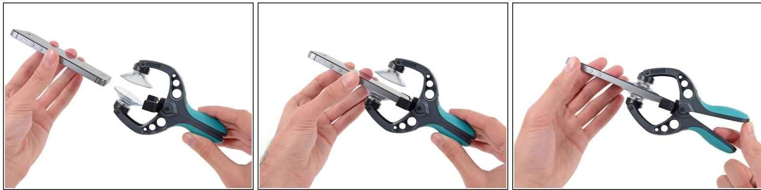
**(i)** The next two steps demonstrate using the [iSclack](#), a great tool for safely opening the iPhone 5 that we recommend for anyone doing more than one repair. **If you aren't using the iSclack, skip to Step 6.**
