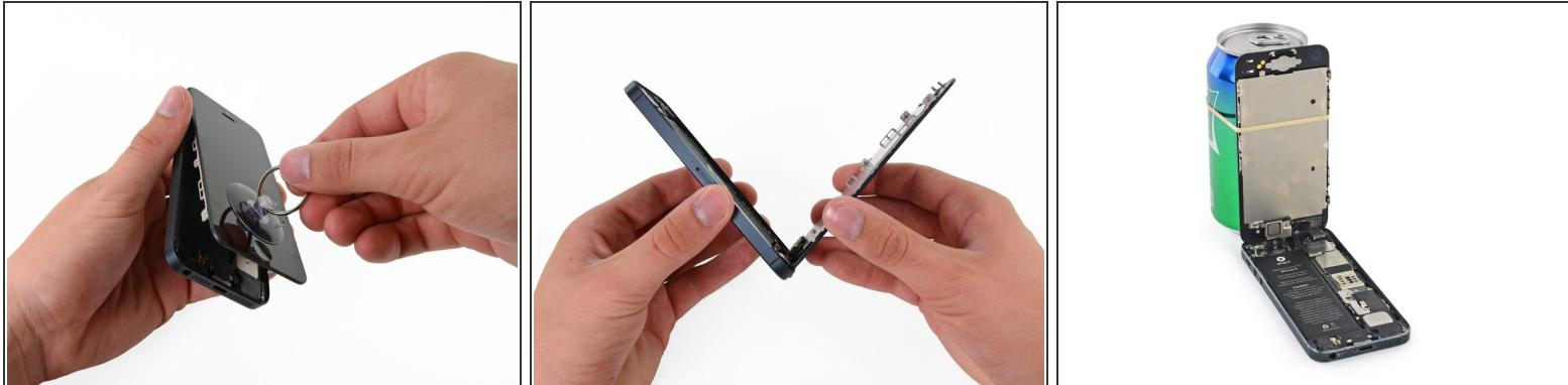
! Do not try to completely remove the front panel assembly from the rear case, as there are several ribbon cables still attached at the top of the iPhone.
