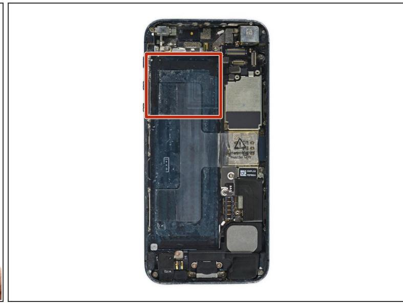
**⚠** Use the plastic opening tool to **gently** pry the battery up, **only at the outside edge of the phone**. Prying anywhere else, especially near the logic board, **may result in damage to the logic board**.
