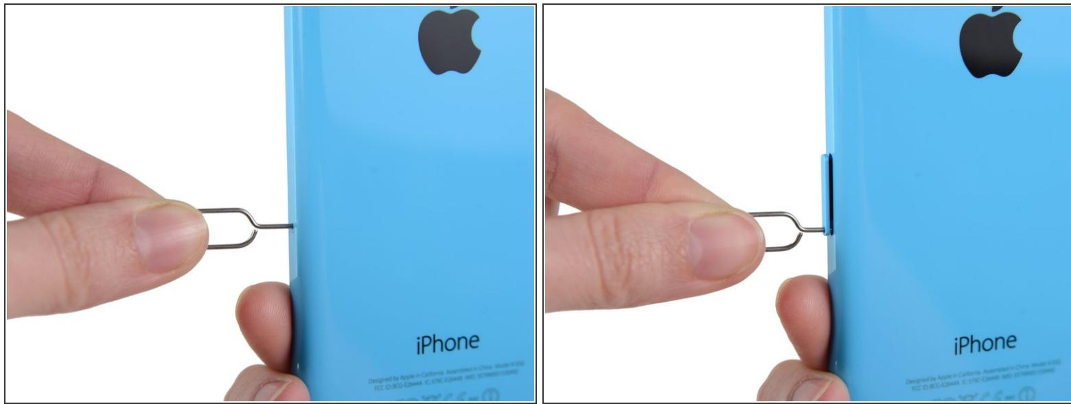
*(i)* Shut your phone down completely before removing the SIM card and tray.
