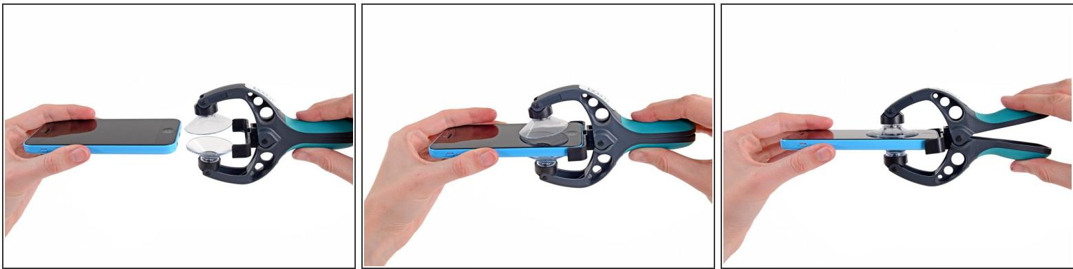
ⓘ The next two steps demonstrate using the [iSclack](#), a great tool for safely opening the iPhone 5c that we recommend for anyone doing more than one repair on an iPhone 5, 5s, or 5c. **If you aren't using the iSclack, skip to [Step 5](#).**
