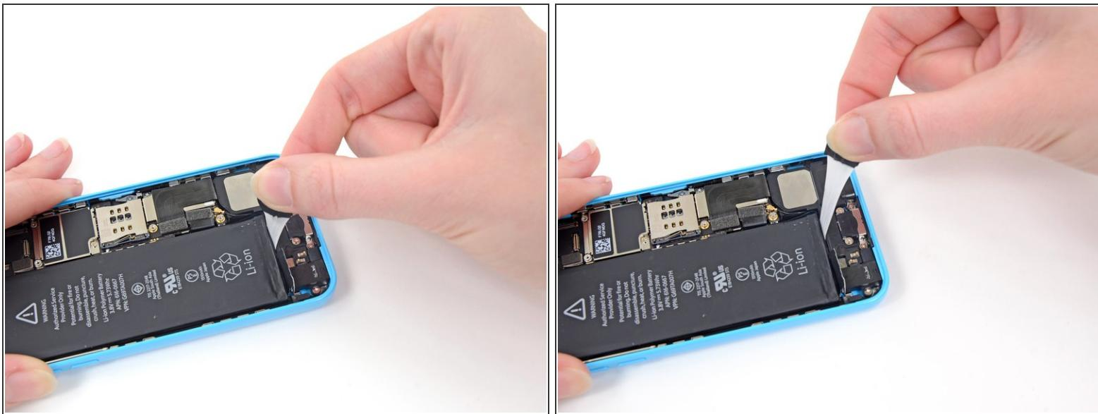
**⚠** Try to keep the strips flat and unwrinkled during this procedure; wrinkled strips will stick together and break instead of pulling out cleanly.
