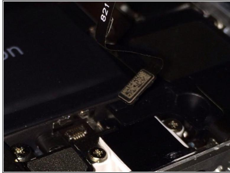
! After using spudger or suction cup to lift screen. Be careful not to pull screen completely up. The touch id sensor flex cable is attached near the home button. There is a small metal clip that needs to be carefully pry'd off before removing flex cable connector.
