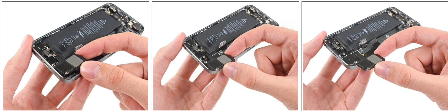
*(i)* The speaker has a small peg that slides into a slot beneath the home button cable socket.
